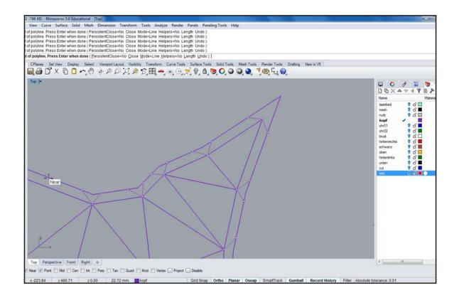
Use \_DupEdge to duplicate all edges that are to be fold. Do not duplicate borders which will be cut. Repeat these steps until all elements are finished. Use \_SelDup or \_SelDupAll to check for duplicate lines.
