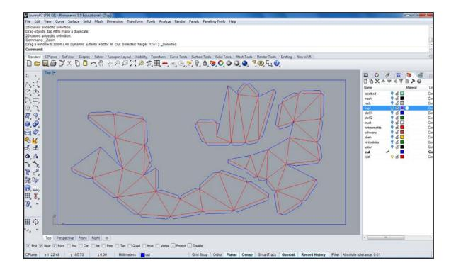
Many glue joints will be double since it is tedious to identify them prior to fabrication. This 15 can only be done by comparing their length manually using the command \_Length. Therefore unnecessary glue joints might have to be removed during assembly using scissors or a knife. The pieces can then be put together.
