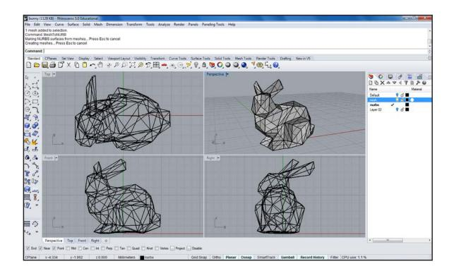
Depending on the complexity of the geometry it might not be developable in one piece. The command \_UnjoinEdge can be used in order to break the object into several smaller parts. The command needs to be repeated until all parts can be unrolled without overlaps as shown in the following step.
