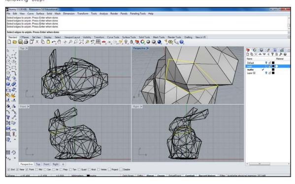
The Command \_UnrollSrf will then flatten the developable surfaces onto the X-Plane. Select 'Explode=No' to keep the parts connected.
