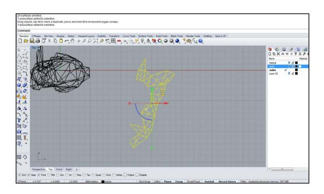
The previous steps need to be repeated until all parts are unrolled. Organizing the different parts into separate layers helps to identify them again later. Using the command \_TextObject they can also be labeled to simplify assembly.
