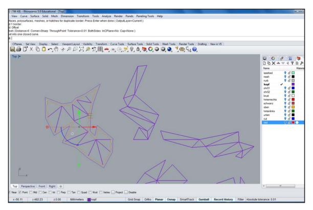
Use the shifted border as a guide to manually draw the gluing joints. When finished erase the previously created border.
