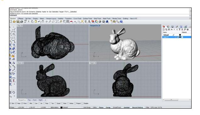
Use \_Mesh to transform NURBS geometry into MESH geometry. Fewer polygons will result in a coarser mesh, more polygons in a more detailed representation. More info on meshes can be found here: http://wiki.mcneel.com/rhino/meshfaqdetails
