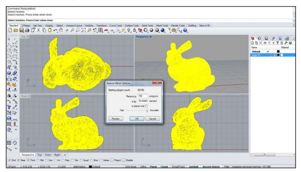
Check the appearance of the geometry. Turn on control points (\_PointsOn) to adjust mesh polygons manually and - if desired - transform the geometry.
