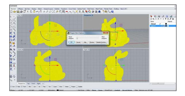
Use \_ReduceMesh to adjust the amount of polygons. Meshes of about 120 - 150 polygons can be easily manufactured. A higher number will result in a higher 'resolution' but also more complex fabrication and assembly.
