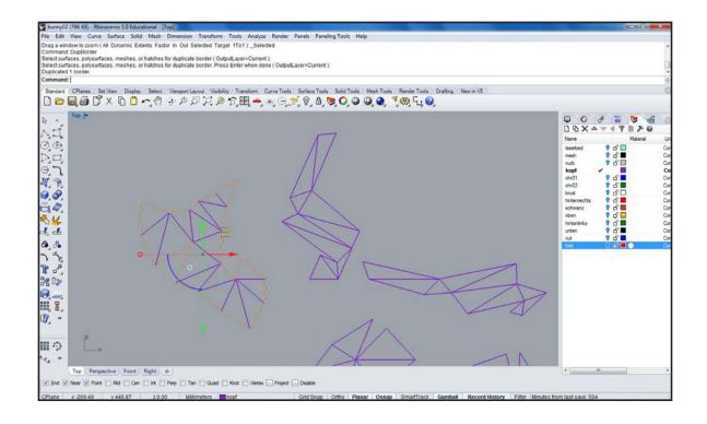
Use \_Offset and choose as 'Distance' a number large enough for the gluing joints. Depending on the model size 3 - 8 mm should be sufficient.
